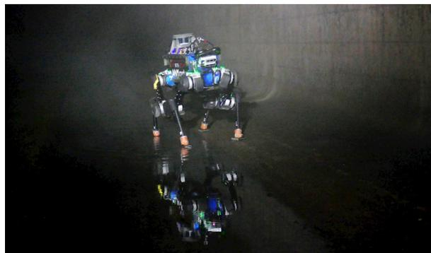
**Fig. 1** An ANYmal robot (Hutter et al. (2016)) in a sewer with two feet in a slippery, wet depression and two feet in a dry, elevated area. With prior information about terrain type and geometry, it is possible for the robot to localized in the world using only touch. This would be extremely useful in dark and foggy environment (Image courtesy of RSL/ETH and from Kolvenbach et al. (2020)).
