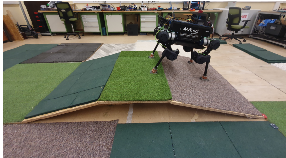
Figure 2: The ANYmal robot walking over the prepared terrain course to collect dataset.
