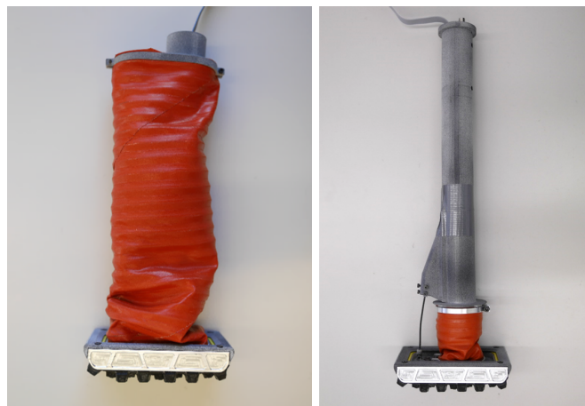
(a) Linear ankle with mounted bellow. For testing purposes with a shorter shank.
