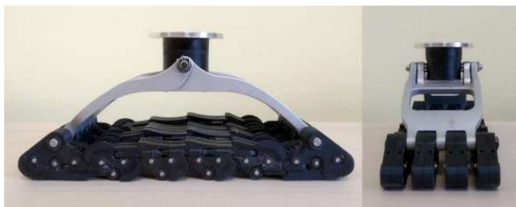
Figure 1: Side and front photos of the passive THING adaptive foot.
