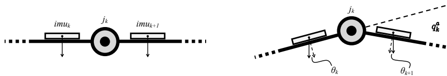
Figure 8: Simple illustration of revolute joint with two IMUs on the adjacent links.
