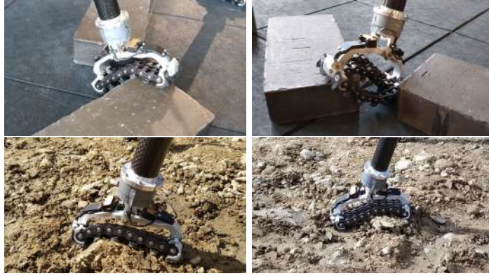
Figure 4: Examples of feet deformations and interactions with different obstacles and terrains.
