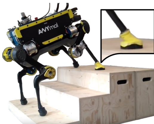
Fig. 1: The adaptive foot allows the quadrupedal robot ANYmal to adapt to the geometry of the ground and gather information about the ground inclination. It features a larger contact area than comparable ball-shaped feet providing better impact absorption and force distribution. The measured contact forces allow for reliable contact detection and permit to optimize the force distribution among the feet.
